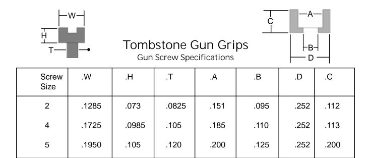
Tombstone gun grip screw kits consist of a screw, a ferrule (illustrated above) and a press-fit nut which has the same diameter and height as the ferrule. The screws are of the slotted fillister head type. Number 2 has 56 threads/inch (2-56). Number 4 has 40 threads/inch (4-40). Number 5 also has 40 threads/inch (5-40). The ferrule for the 2-56 screw will also work with most Fillister slotted head 3-48 screws (the nut would need to be re-tapped for the larger thread size).
